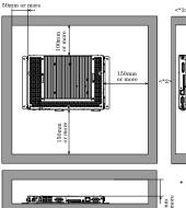
When installing to a 35mm-wide space betw walls
